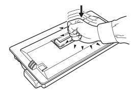
**6** Thoroughly shake the toner container (in the direction of the arrows) ten times or more to loosen and mix the toner inside.
